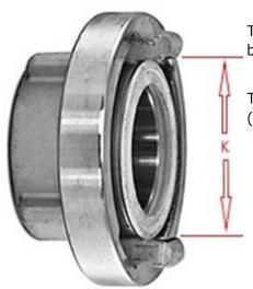
To determine the correct size of a STORZ coupling face a measurement between the two lugs on the coupling face as shown (left) must be taken.
